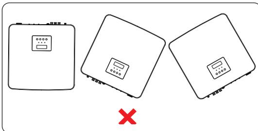
Figure 7-2 Incorrect installation
