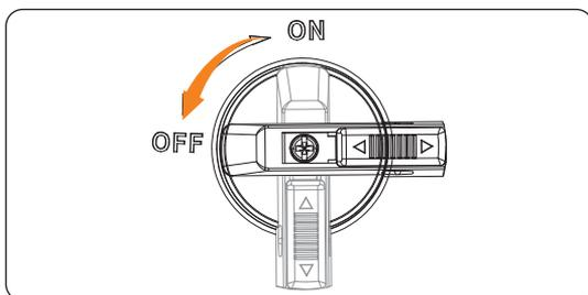
Figure 9-7 Turning off the DC switch
