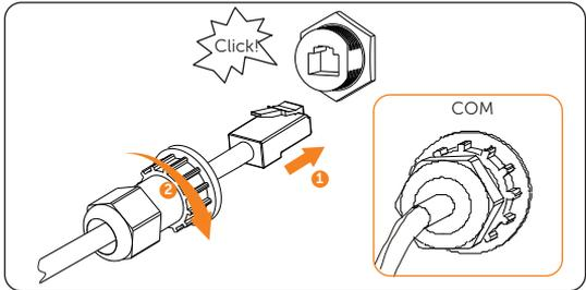
Figure 8-33 Connecting to COM terminal
