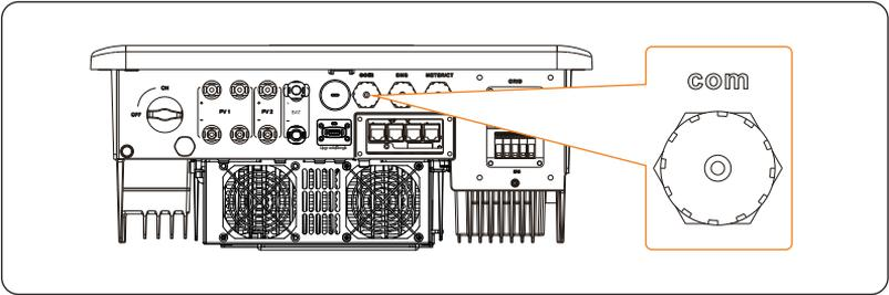
Figure 15-5 Connection terminal for Adapter Box G2
