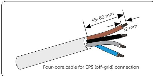
Figure 8-9 Stripping the EPS (off-grid) cable
