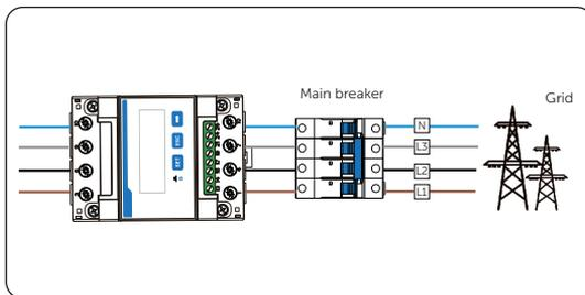
Figure 15-27 Connecting direct-connected meter to the grid
