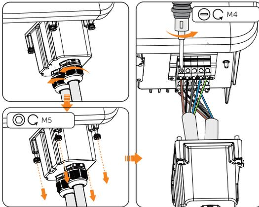
Figure 13-4 Disconnecting the AC connector
