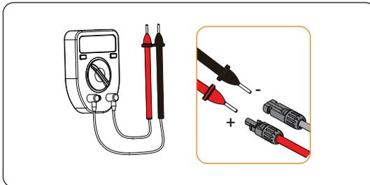
Figure 8-21 Measuring the voltage of PV connectors
