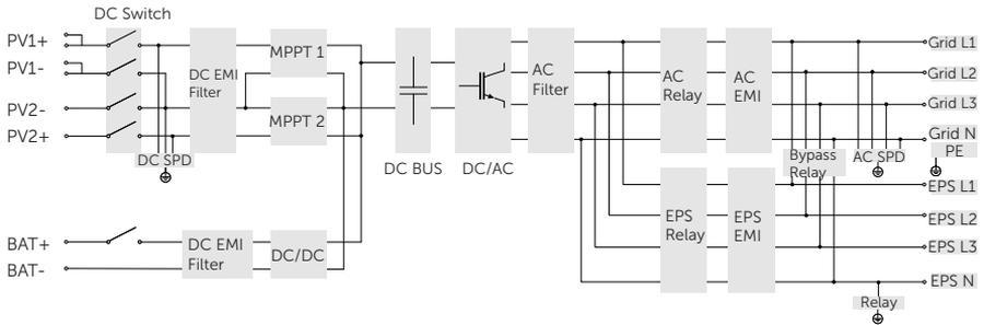
Figure 2-5 Circuit Diagram for X3-Hybrid G4 series inverter
