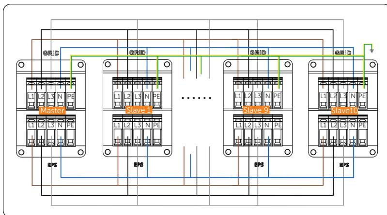
Figure 15-15 Power cable wiring with X3-PBOX device
