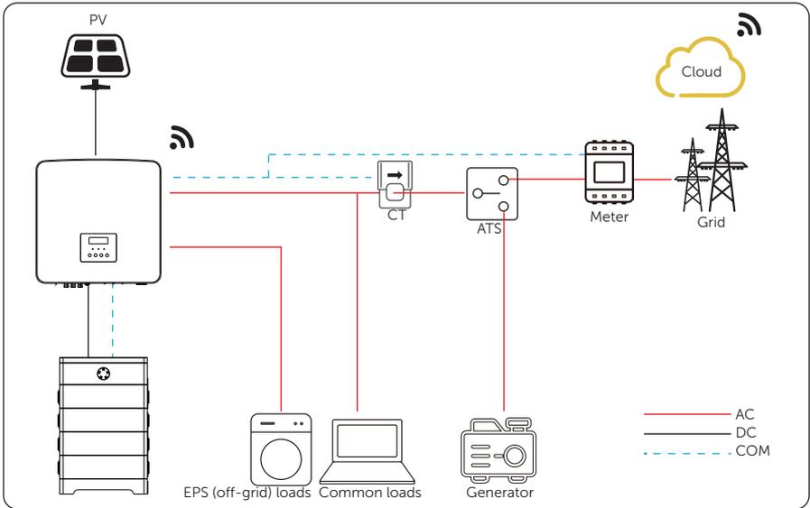
Figure 15-1 ATS control wiring diagram
