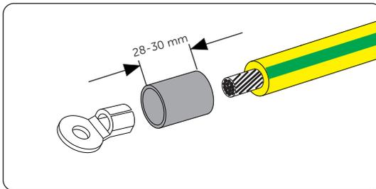
Figure 8-4 Installing the tubing and OT terminal
