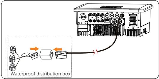
Figure 15-23 Connecting the inverter to the CT
