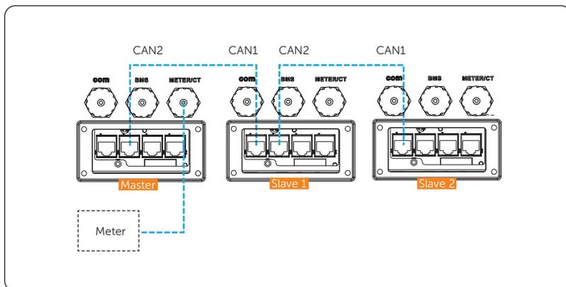
Figure 15-18 Communication wiring without X3-PBOX device
