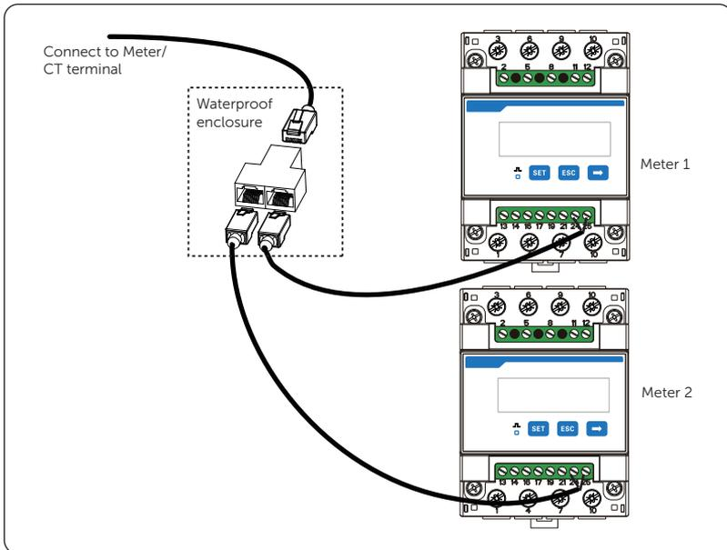
Figure 15-39 Connecting to RJ45 splitter adapter
