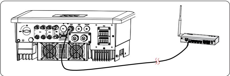
Figure 15-12 Connecting to DataHub
