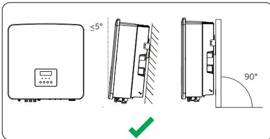
Figure 7-1 Correct installation
