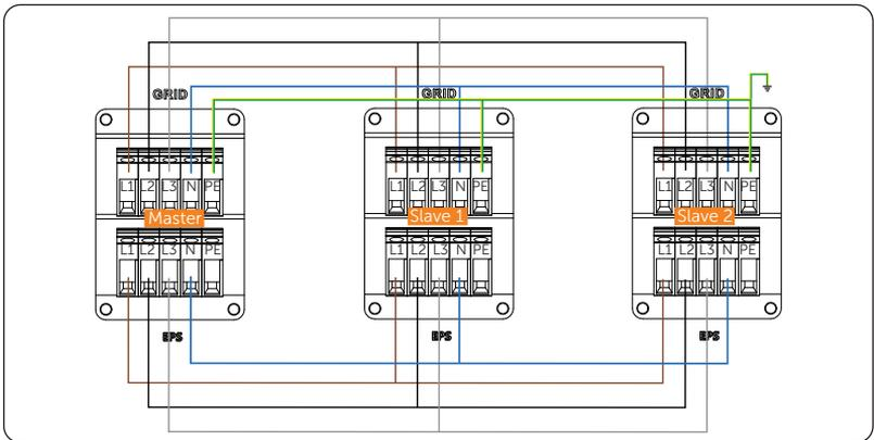
Figure 15-17 Power cable wiring without X3-PBOX device
