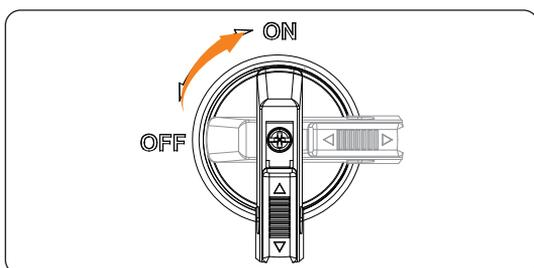
Figure 9-6 Turning on the DC switch
