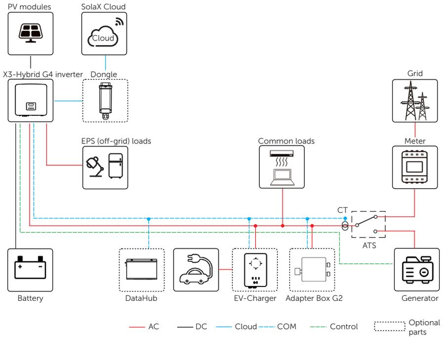
Figure 3-1 System diagram
