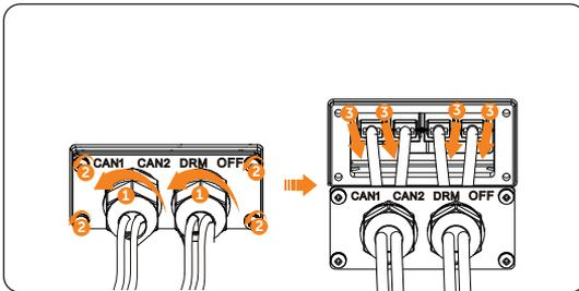
Figure 13-6 Disconnecting the CAN1 / CAN2 / DRM / OFF cable
